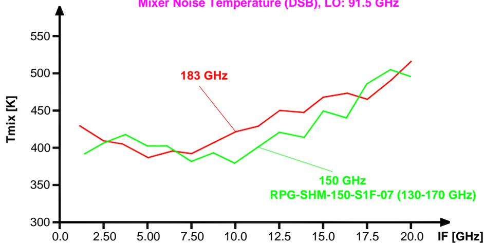
**Fig.2.2c: RPG-LHATPRO 183 GHz SHM performance over IF bandwidth.**
