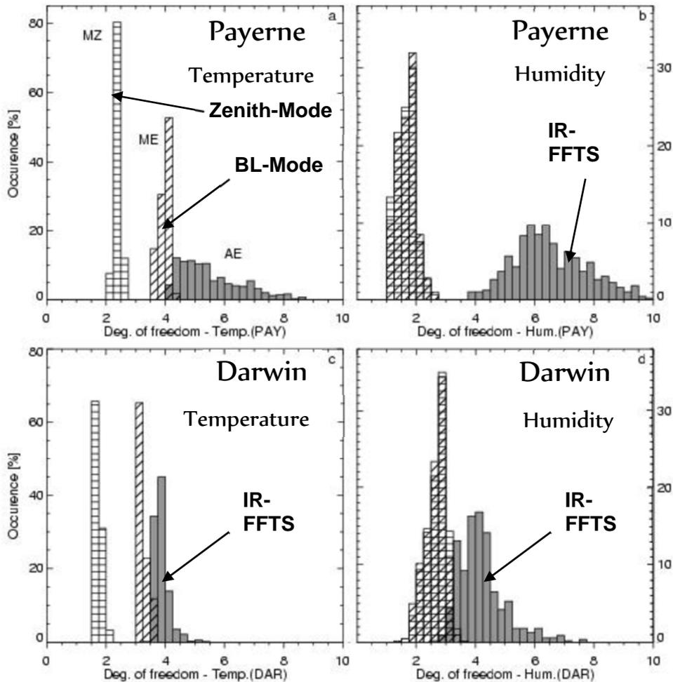
**Fig.3.6: Comparison of degrees of freedom for different scanning modes (Boundary Layer scanning BL-Mode and Zenith Observation Mode) and data from an infrared FFTS spectrometer (to be ignored in this context).**
