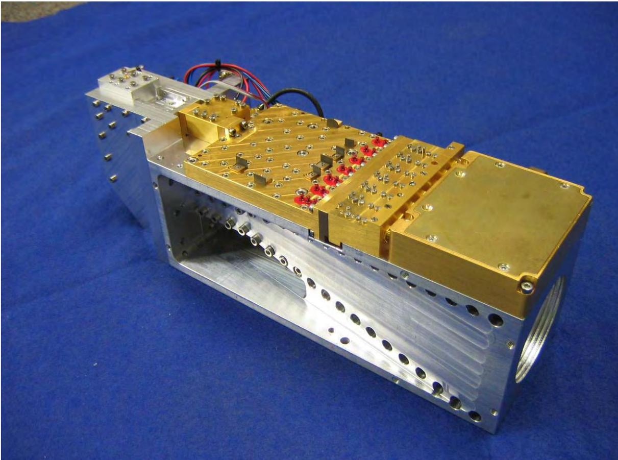
**Fig.2.3: Temperature profiling direct detection filter bank receiver mounted to the 50-60 GHz corrugated feedhorn. Receiver size: 72 x 200 x 15 mm<sup>3</sup>.**
