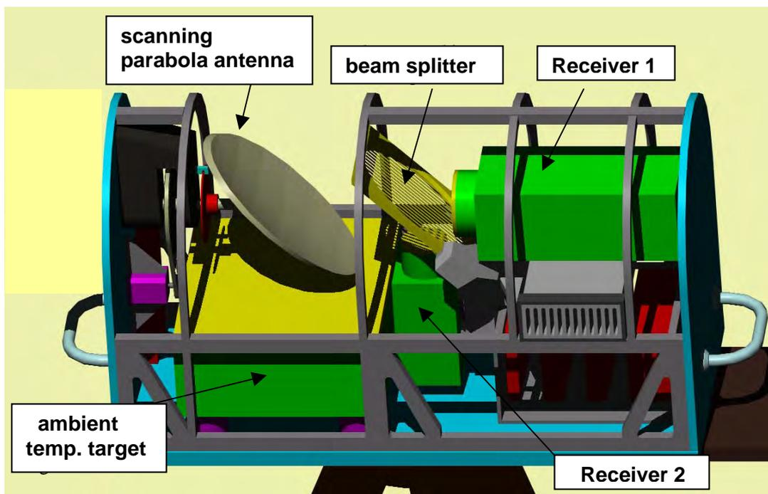
**Fig. 2.1: Schematic internal structure of un-polarized RPG radiometers.**
