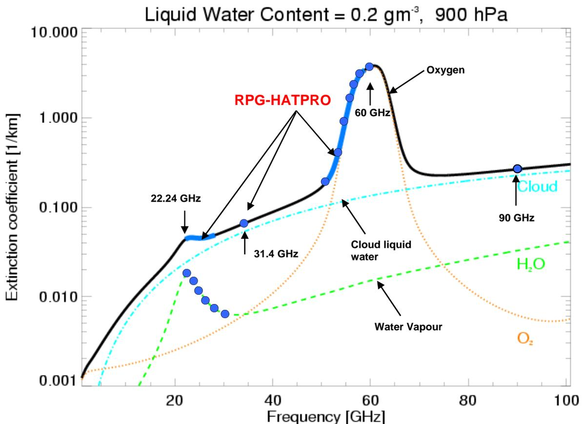
**Fig.3.1: Spectral features used for microwave atmospheric profiling**
