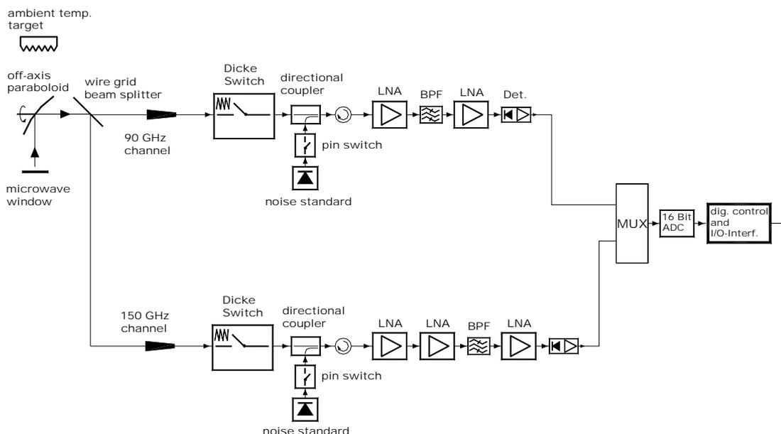
**Fig.2.2e: RPG-150-90 precision LWP radiometer receiver layout. The system is equipped with a full set of calibration standards (noise diode + Dicke switch).**
