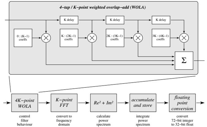
**Fig. 6.** Block diagram of the polyphase filter bank (PFB) signal processing pipeline. The PFB not only produces a flat response across the passband, but also excellently suppresses out-of-band signals.
