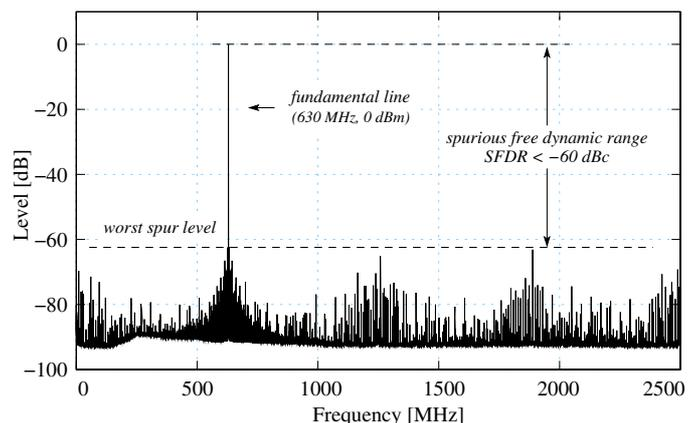
**Fig. 9.** Measured spurious free dynamic range (SFDR) of the XFFTS with E2V's 10-bit 5 GS/s ADC for a fundamental line injected at 630 MHz. Over the whole 2.5 GHz bandwidth the SFDR is below  $-60$  dBc, perfectly confirming the vendor specifications for this ADC.
