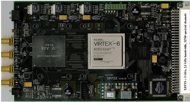
**Fig. 4.** XFFTS board that uses E2V’s fastest  $4 \times 1.25$  GS/s 10-bit ADC and the high-performance Xilinx Virtex-6 LX240T FPGA. By applying time interleave techniques, the four 1.25 GS/s ADCs can be combined into two 2.5 GS/s or one 5 GS/s converter. The XFFTS allows analyzing an instantaneous bandwidth of 2.5 GHz with 32k spectral channels. Depending on the processing set-up and the input signal level, the board consumes 20–25 Watt.
