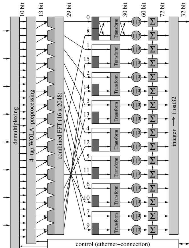
**Fig. 7.** 32k spectrometer design with a combined 32768-points FFT ( $16 \times 2048$ ), running on a Xilinx Virtex6 LX240T FPGA. Data width grows by  $\log(4) + 1$  bits in four-tap WOLA, by  $\log(32768) + 1$  bits in 32 768-points FFT, by 1 bit during channel transformation and is doubled by squaring.
