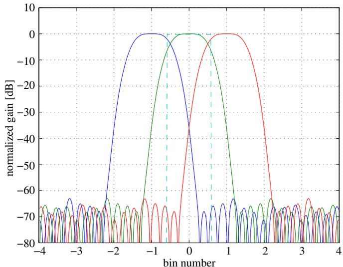
**Fig. 8.** Frequency response of the polyphase filter bank signal processing pipeline. The diagram shows three adjacent frequency bins in logarithmic scale measured with the 32k channel XFFTS. The dashed lines illustrate the equivalent noise bandwidth (ENBW) for the corresponding spectral bin.
