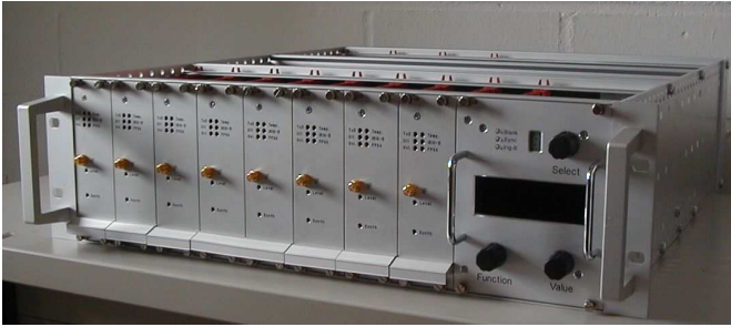
Fig. 3 Photograph of our 19 inch FFTS-crate, equipped with eight FFTS-boards and one FFTS-controller unit. The modular concept allows combining multiple crates to build large FFTS arrays.
