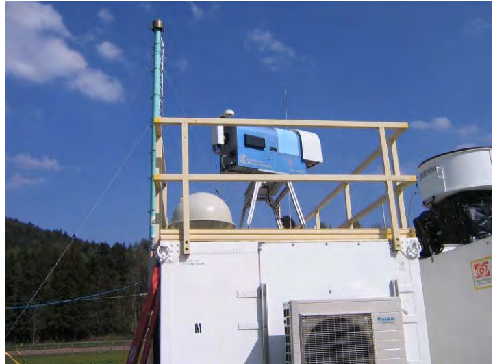
Figure 2.39: A HATPRO instrument with azimuth positioner during full sky scan operation at the US ARM mobile facility.
