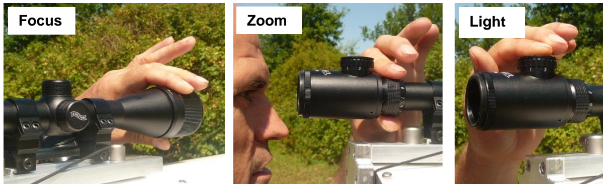
Figure 31: Adjustment of the MWS/LAS alignment telescopes.
