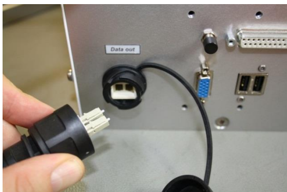
Figure 27: Setting up the fibre-optical cable for data transfer.
