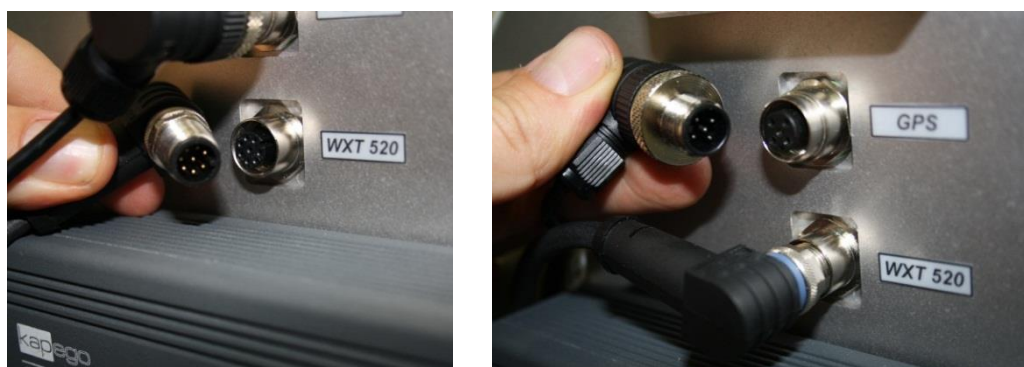
Figure 16: Connecting GPS clock and weather station.
