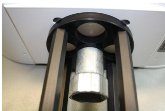
Figure 23: Double base plate and mounting adaptors for LAS transmitter and receiver.
