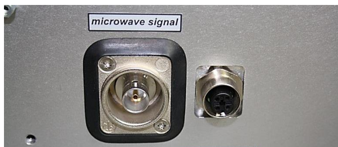
Figure 25: BNC connector (left) to read the RPG-MWSC-160 detector voltage (only for diagnosis).
