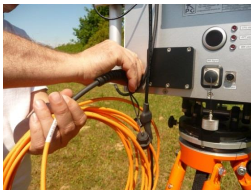
Figure 27: Setting up the fibre-optical cable for data transfer.
