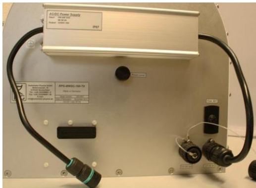
Figure 9: Left: AC power supply mounted to RPG-MWSC-160 transmitter, Right: 50 m power cable.
