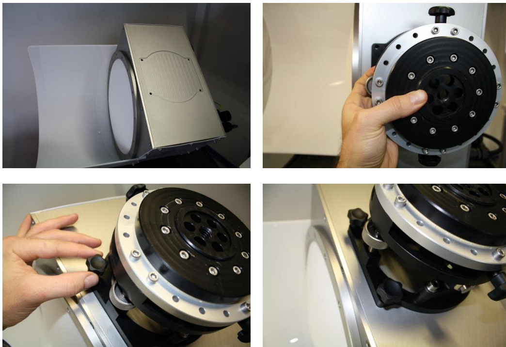
Figure 20: No tools are needed to fasten the alignment unit to the RPG-MWSC-160 units.
