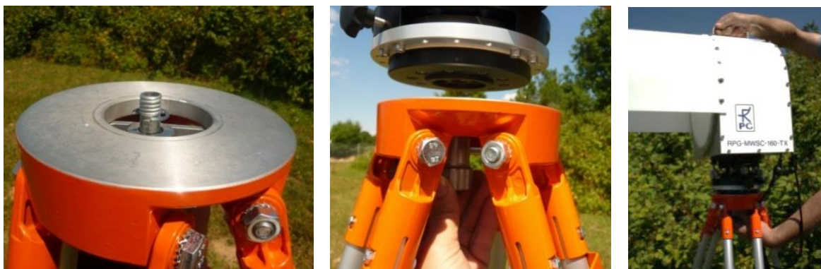
Figure 21: Fasten center bolt to mount RPG-MWSC-160 units on a tripod (single configuration).
