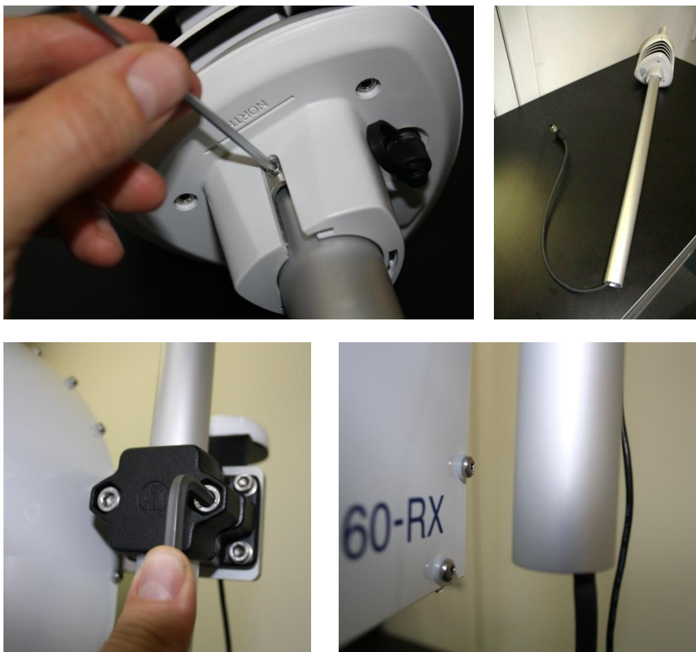
Figure 15: Mounting the weather station Vaisala WXT-536. A: Fix the station on top of the pole. The "North" arrow has to be aligned with the instrument's side wall. B: Station, mounting pole and connecting cable. C: Use Allan key to mount the pole to the RPG-MWSC-160 receiver. D: Take care that the pole ends well above the receiver's bottom plate level.
