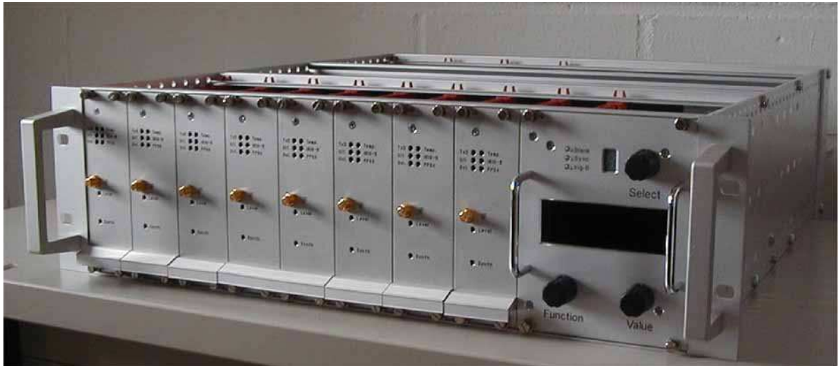
19" AFFTS crate equipped with 8 FFTS boards and one FFTS controller (right side)
