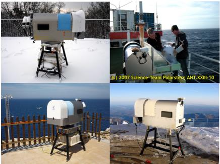
In a similar approach, the absorption line of the water vapour molecule at 22.235 GHz can be used to asses the mixing ratio of the water vapour, giving a humidity profile. Cloud water is also detectable by inspecting frequencies which are either in or out of the water vapour line, this discriminating the influence on such channels by either liquid water or the gaseous form of water vapour. Mathematical retrieval procedure are used to invert this (usually ill-posed) information problem.
