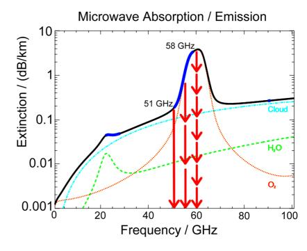
water, rain) is having an emission at all frequencies of the spectrum. Different atmospheric conditions (temperature profile, humidity profile, clouds) will lead to different contributions, which are all received together. Still, there is a kind of "fingerprint" of an atmospheric state in the way the multi-channel signature would be impacted.
