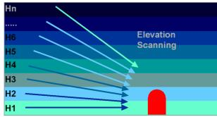
(zenith) pointing. At the smallest elevation angles, the radiation is only originating from the lowest level of the atmosphere and thus giving a temperature information of only this layer. Scanning to the next elevation, the beam is intersection more layers (but still has a limited reach), so the temperature is a mixture of two layer temperatures. With the first temperature
