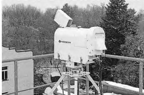
FIG. 1. The microwave profiler TP/WVP-3001.
