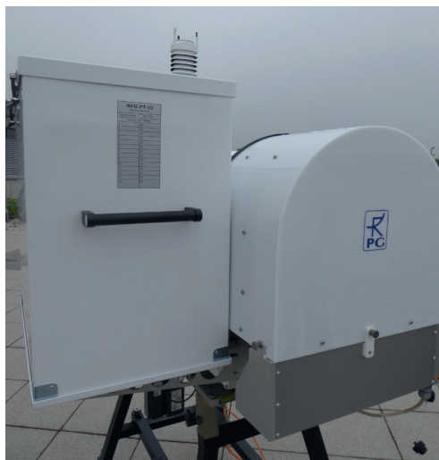
RPG-HATPRO-G5 radiometer during the absolute calibration procedure with RPG's LN2-cooled target PT-V2.
