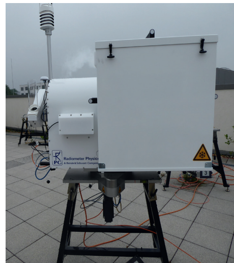
RPG-HATPRO-G5 radiometer during the absolute calibration procedure with RPG's LN2-cooled target PT-V2.
