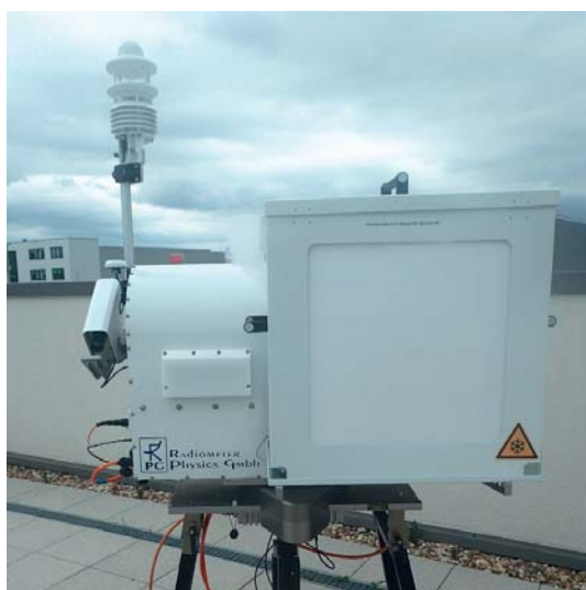
RPG-HATPRO-G5 radiometer during the absolute calibration procedure.
