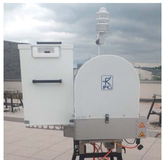
RPG-HATPRO-G5 radiometer during the absolute calibration procedure.
