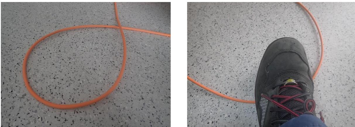
**Fig.2.8.1: Avoid loops in the fiber optics cable. The curvature radius should not be less than 5 cm. Crossings of cables can lead to cable damage when stepping on it.**
