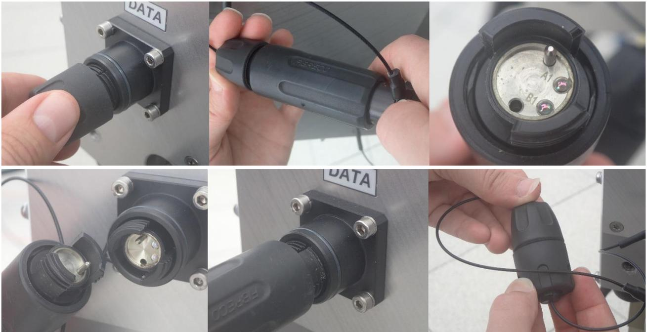
**Fig.2.5.6: Connecting the fiber optics data cable.**
