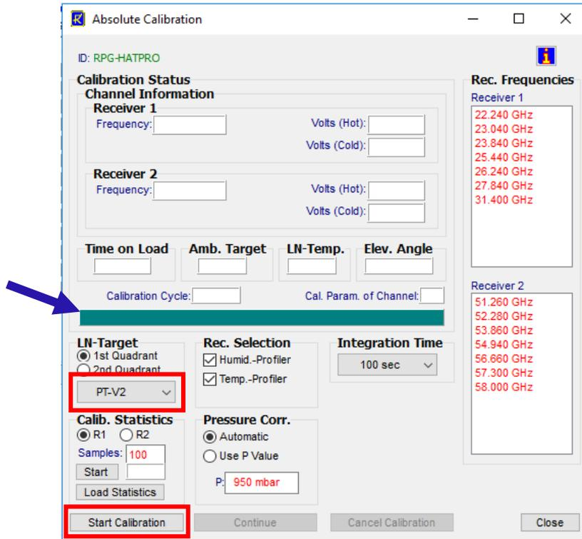
**Fig. 4.3.6:** Choose the target PT-V2 from the drop-down menu. The button **Start Calibration** starts the absolute calibration procedure. The dew blower will switch to high-speed mode and the heater will be activated. This prevents condensation of water vapor on the target observation window facing the radiometer. Follow the instructions displayed in the message line (indicated by a blue arrow).
