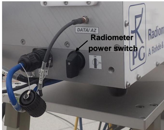
**Fig 3.1.1: Radiometer power switch in OFF position.**
