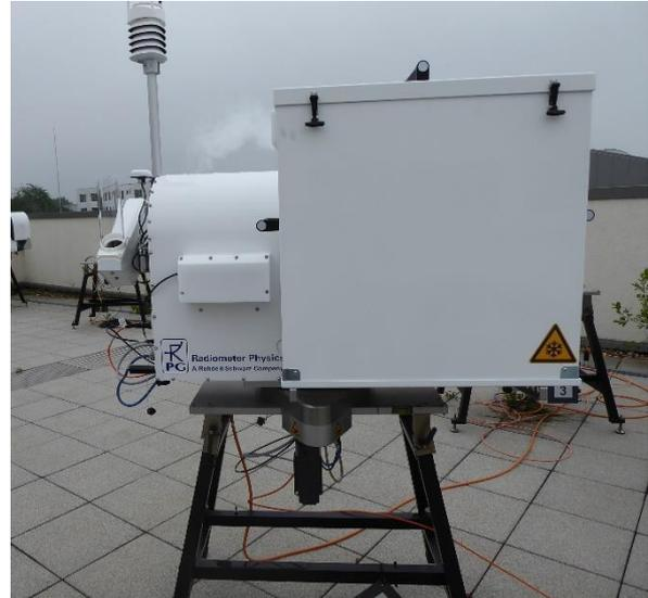
**Fig. 4.3.5:** Place the target on the table. Make sure that the target's sidewall marked with "R1" is facing the radiometer.
