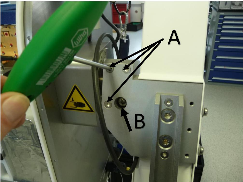
**Fig.2.6.13: For the motorized IR-Option (Option IRR-B), the IR radiometer is mounted with three M4 screws (A). NEVER touch the screw in (B). It has been adjusted to an elevation axis tilt accuracy of 0.3°. By loosening (B), this adjustment is lost.**
