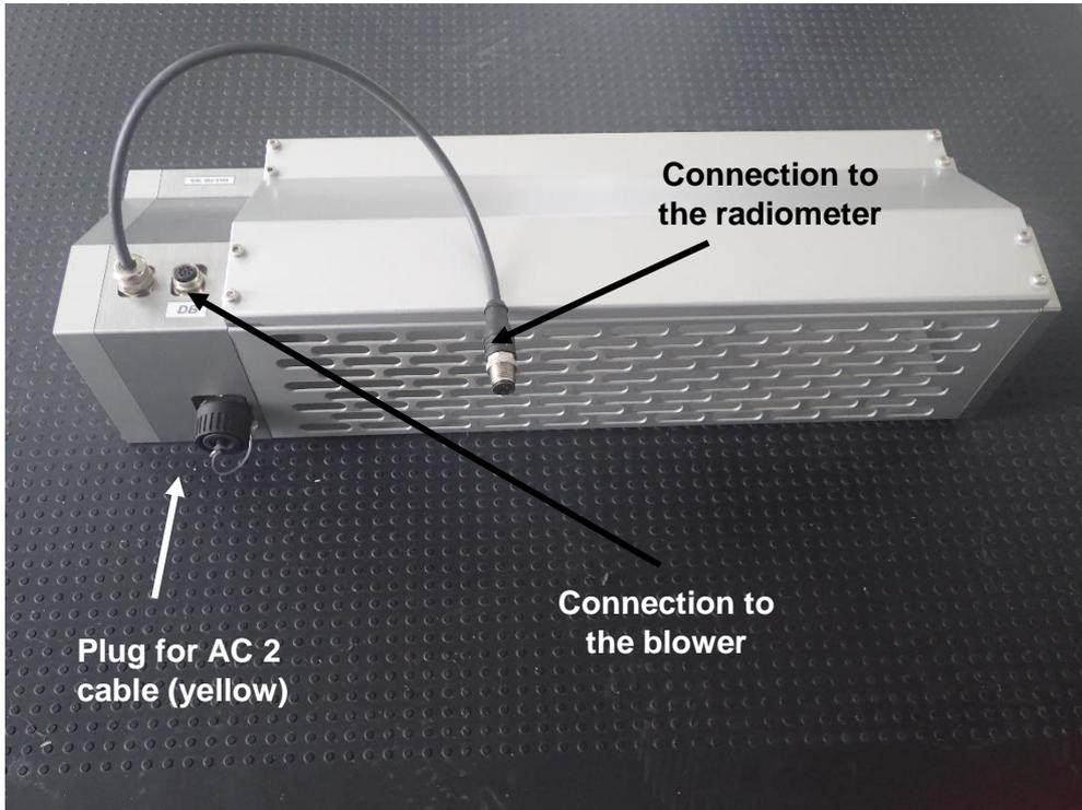
**Fig.2.6.3: Dew blower heater module with mounting points.**
