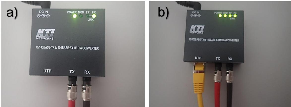
**Fig.2.7.3: 2 line fiber optics to LAN-TCP/IP converter.**
