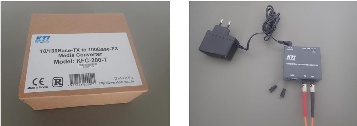
**Fig. 2.7.1: Fiber-to-LAN-TCP/IP converter.**
