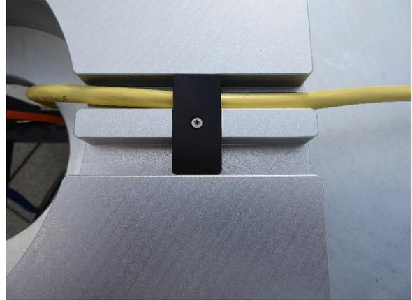
**Fig.2.4.8: Mounting the cables into the cable channels.**
