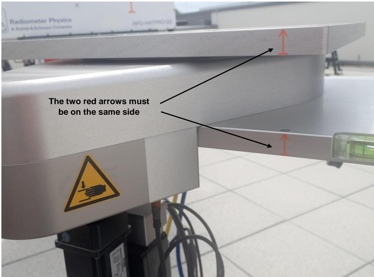
**Fig.2.4.2: Azimuth positioner on the stand's table plate.**
