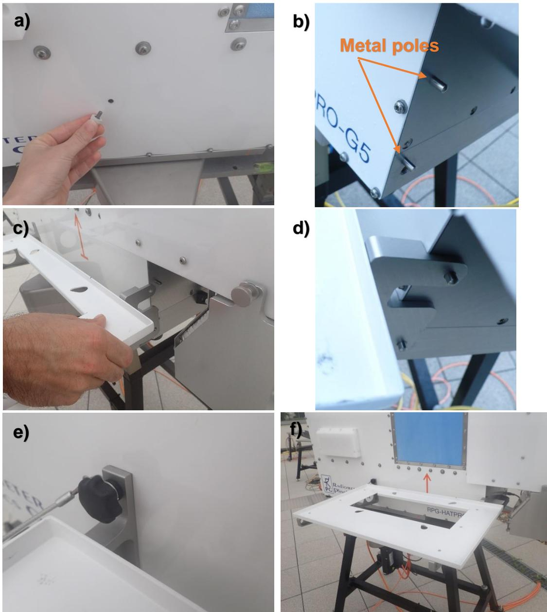
**Fig. 4.3.3: Mounting of the cold load calibration target.**
