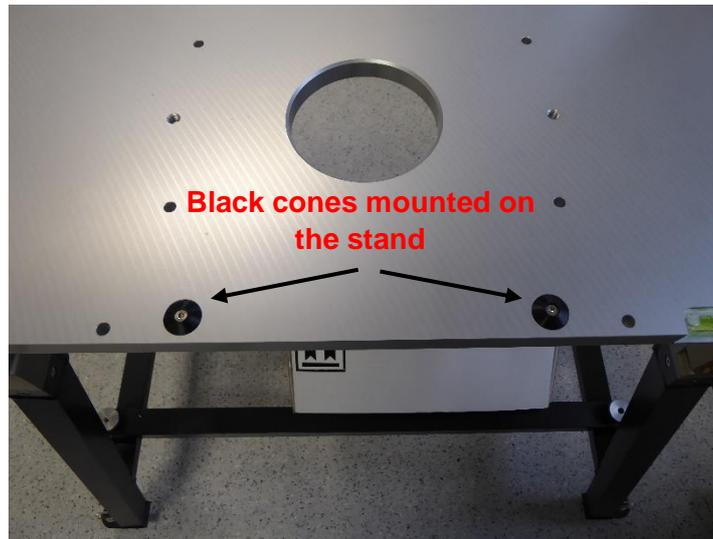
**Fig.2.5.1: Black cones to be mounted only in case of no azimuth positioner**
