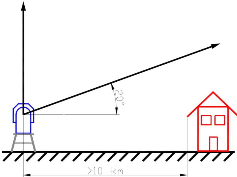
**Fig.2.9.1: Tip curve calibration viewing range.**
