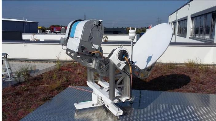
Absolute calibrations using LN2 targets are not taking the losses of the external reflector into account. These losses must be determined in a separate step and for each receiver channel individually.
