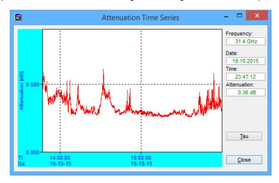
Atmospheric attenuation is calculated along the line of sight at the channel frequencies.
