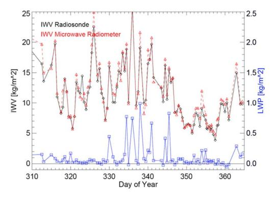
IWV measurements remain accurate even with LWP of 1000 g/m<sup>2</sup>.
