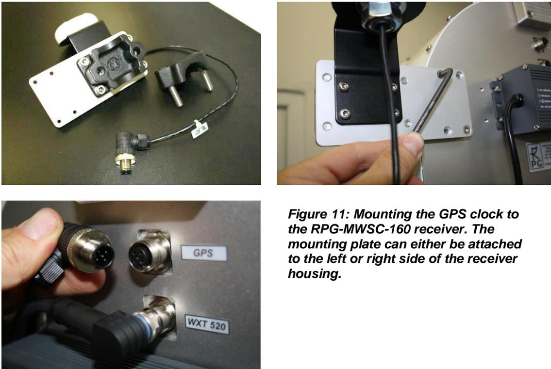
*Figure 11: Mounting the GPS clock to the RPG-MWSC-160 receiver. The mounting plate can either be attached to the left or right side of the receiver housing.*
