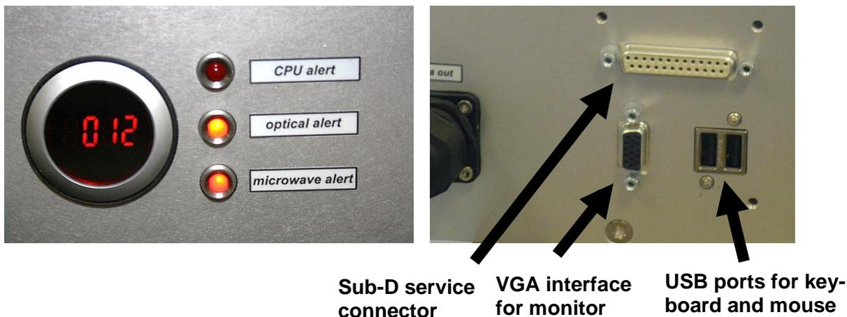
**Figure 2: Left: Signal level and status alerts for the combined system. Right: External ports. Use a Torx key to remove the protecting cap.**
