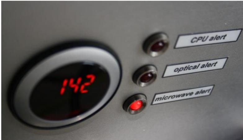
**Figure 26: Receiver signal level display.**
