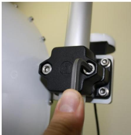
**Figure 12: Mounting the weather station.**
