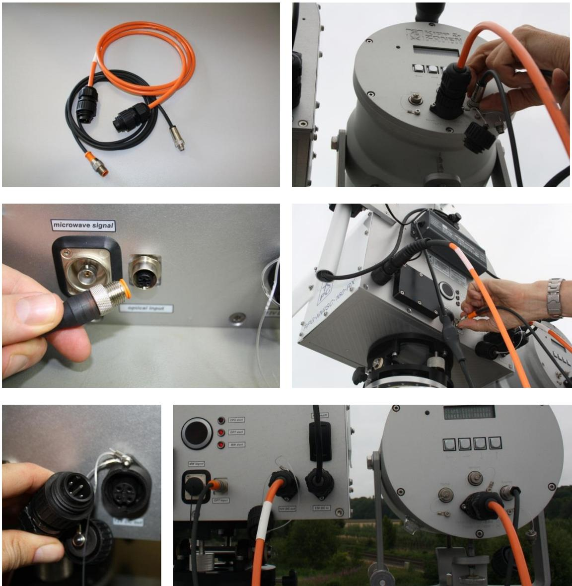
**Figure 20: Example: power and data cables for the Kipp&Zonen Mk-II receiver. On the transmitter side, there is only a power cable.**
