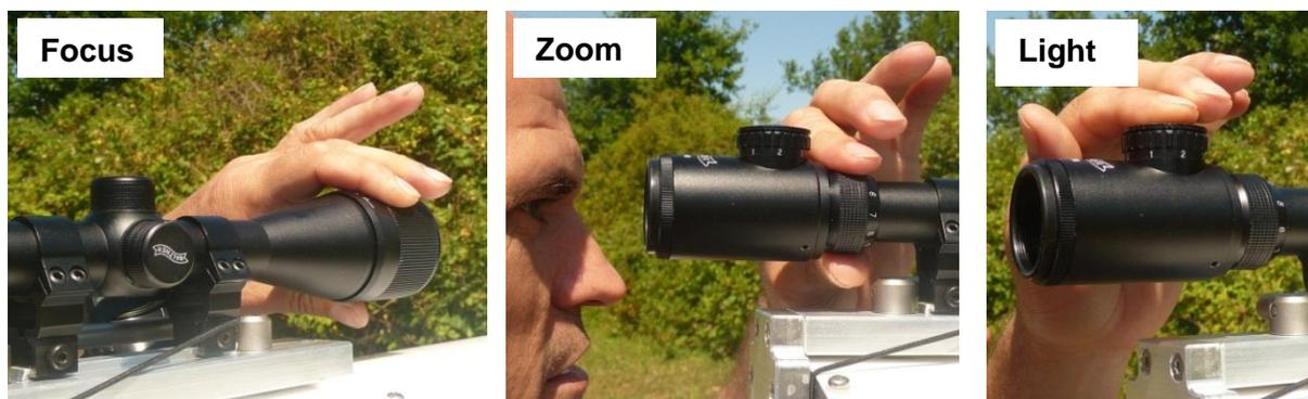
**Figure 25: Adjustment of the MWS/LAS alignment telescopes.**
