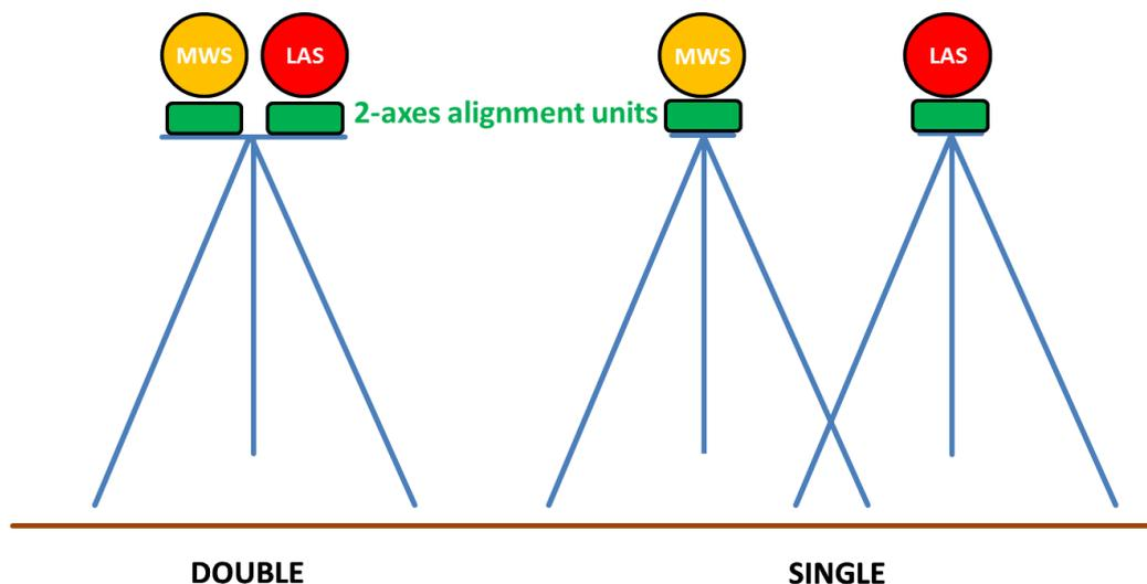
**Figure 6: Mounting options for the combined OMS system.**
