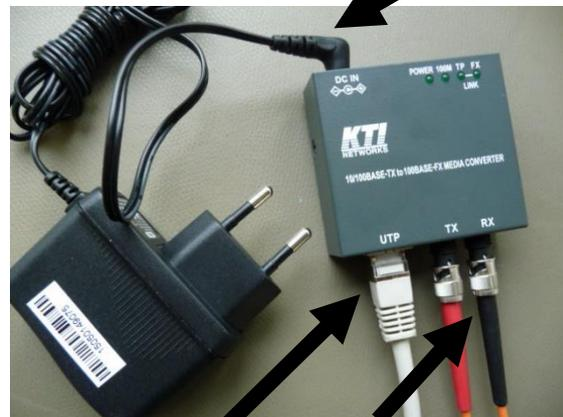
**Ethernet connection    Fibre-optical data cable**
