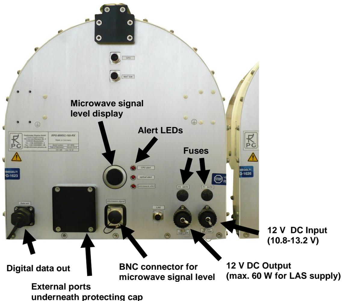
**Figure 1: Rear view of the RPG-MWSC-160 receiver.**
