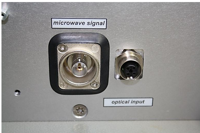
Figure 27: BNC connector to read the RPG-MWSC-160 detector voltage (only for instrument alignment and diagnosis).
