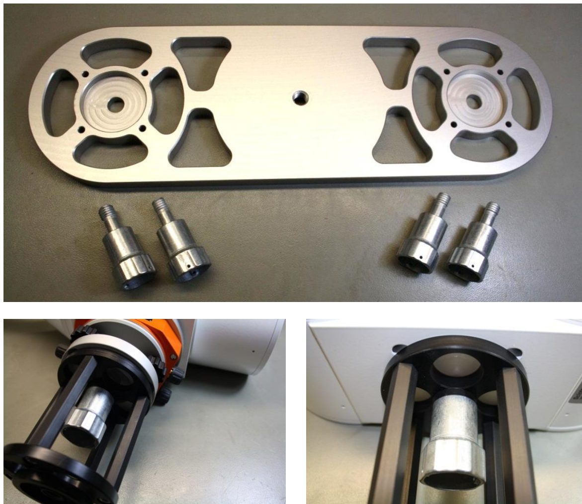
Figure 25: Double base plate and mounting adaptors for LAS transmitter and receiver.
