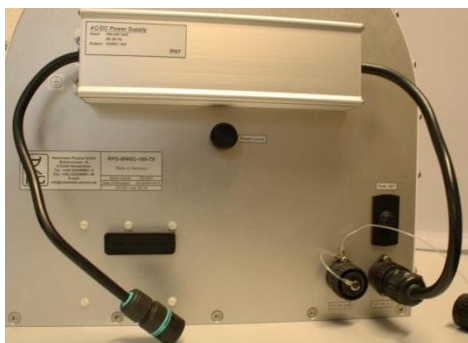
Figure 11: Left: AC power supply mounted to RPG-MWSC-160 transmitter, Right: 50 m power cable.
