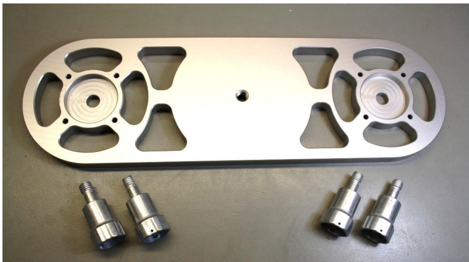
Figure 8: Double base plate for combined mounting of MWS and LAS units.
