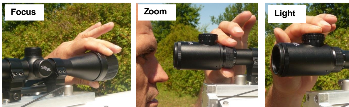
Figure 33: Adjustment of the MWS/LAS alignment telescopes.
