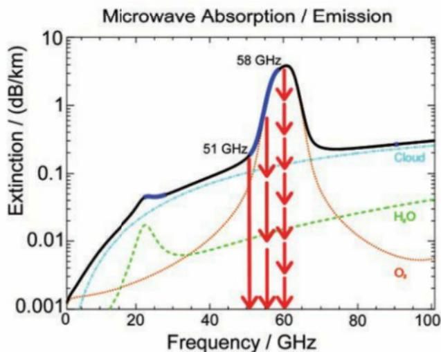
Absorption spectrum in the microwave region with contribution from gases (emission in spectral lines, water vapor: green; oxygen: orange) and from liquid water drops (continuum emission with spectral dependence, blue line)
