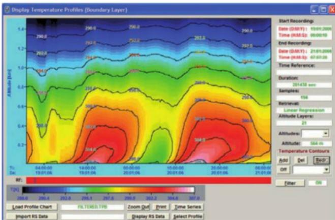
Time series of vertical temperature profile as retrieved from a microwave dual profiler radiometer
