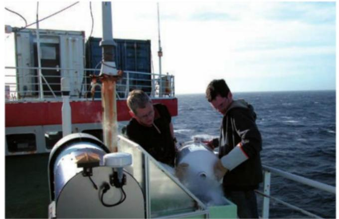
RPG-HATPRO microwave radiometer deployed on German Arctic research vessel 'Polarstern', cruising the Atlantic Ocean. (c) 2007 Science Team Polarstern ANT.XXXIII-10
