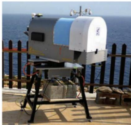
RPG-HATPRO-G2 microwave radiometer deployed at Lampedusa Island, Italy, south of Sicily
