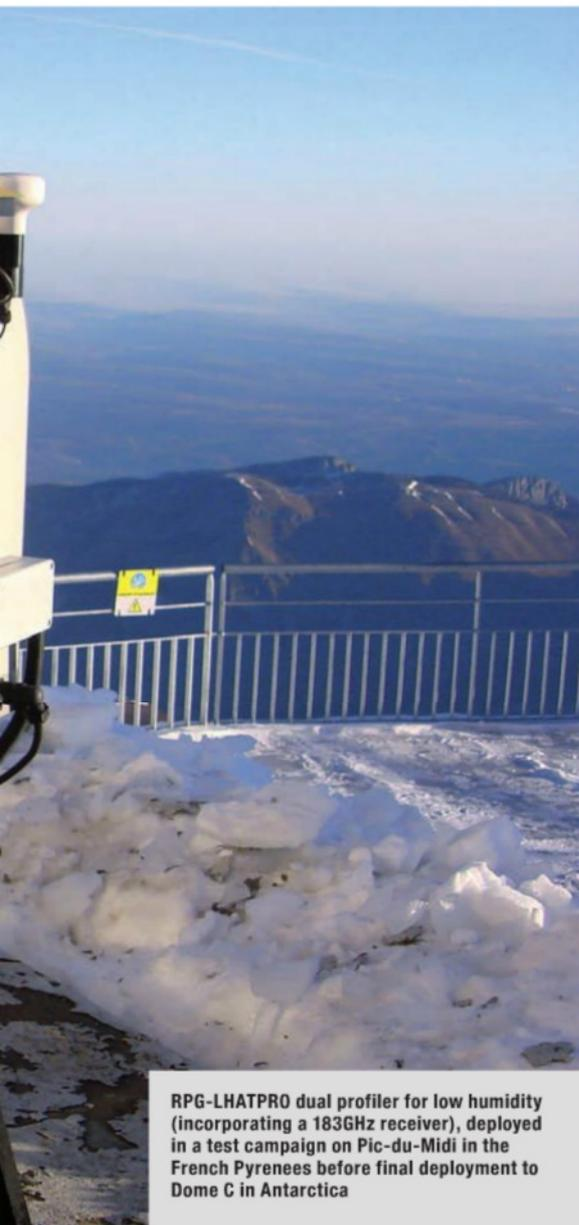
RPG-LHATPRO dual profiler for low humidity (incorporating a 183GHz receiver), deployed in a test campaign on Pic-du-Midi in the French Pyrenees before final deployment to Dome C in Antarctica
