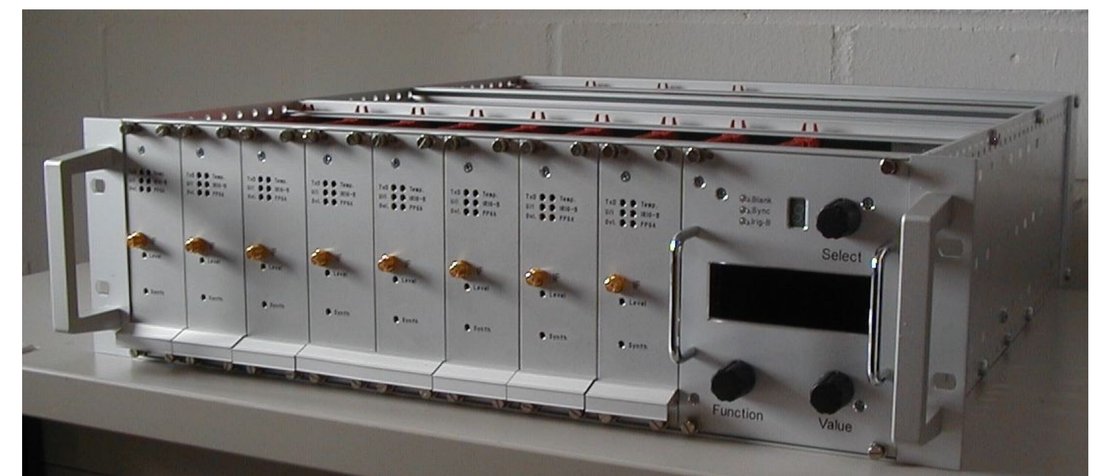
Fig 2 The APEX wideband AFFTS consists of four FFTS-crates, each equipped with 8 FFTS boards and one FFTS-controller. The frequency resolution (equivalent noise bandwidth) for the standard configuration with 1.5 GHz bandwidth and 8192 spectral channels per board is 212 kHz, corresponding to 0,13 km/s at 500 GHz.
