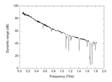
Note: Unless otherwise noted, all specifications are to be treated as "typical" and can be changed without notice. Typical dynamic range dependence on frequency plot for a homodyne setup
