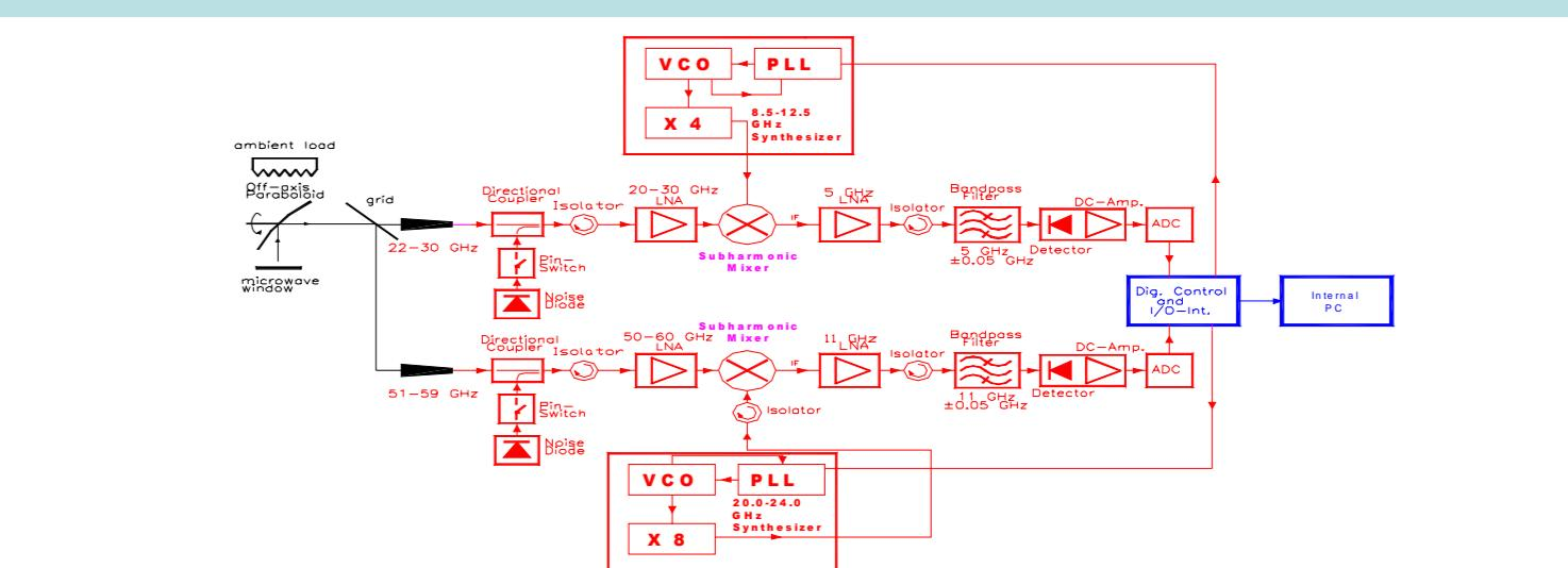
Dual profiler direct detection filterbank receiver:
